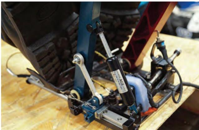
*The GS-15-40-BB-120 undergoes testing. The part's compact dimensions mean that it can be easily integrated into the racecar's existing design.*
