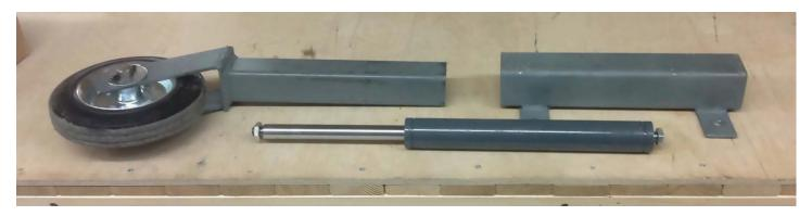
To support the weight of the door, Jorkisch integrated ACE industrial gas springs into the wheel's metal supports.
