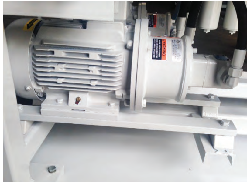
ACE rubber-metal isolators isolate impacts and vibrations from machines and motors, and improve wearing conditions.
