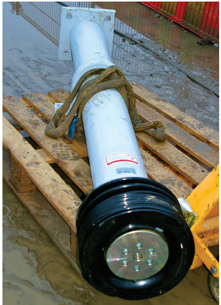
More than 2-m long and weighing in at 320 kg, the special ACE shock absorber features a fixed stop and stroke of 800 mm.
